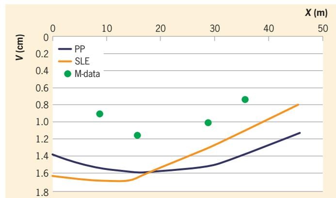
**Figure 10: Results of the PP and SLE calculations – vertical movements, upper edge of the slab in Stage 3 without the effects of the movements relating to the previous stages. Comparison with monitoring data**
