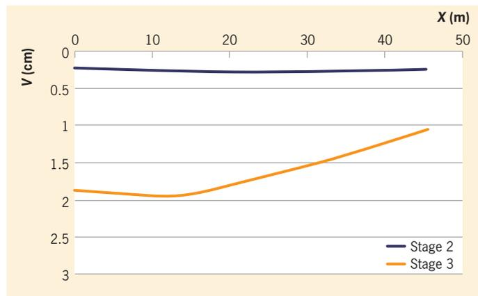
**Figure 7: Results of the SLE calculation – vertical movements upper edge of the slab at Stages 2 and 3**
