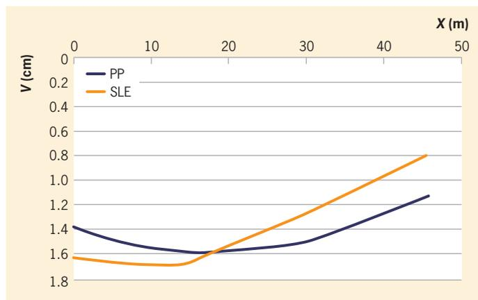
**Figure 9: Comparison of the results of the PP and SLE calculations – vertical movements, upper edge of the slab in Stage 3 without the effects of the movements relating to the previous stages**
