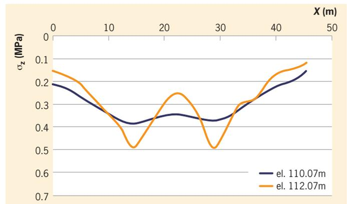
**Figure 8: Results of the PP calculation – Stage 3 vertical stresses on the earth-slab contact interface (el. 112.07m) and 2m deeper (el. 110.07m)**
