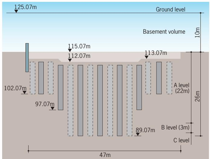
**Figure 3: Cross section of the project (through the minimum width of the slab)**
