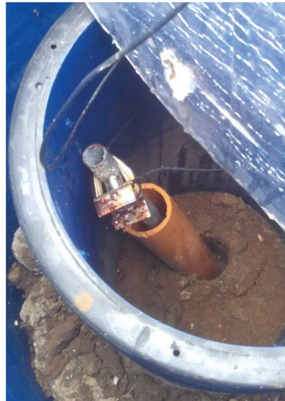
Figures 4a and 4b. Photographs of instrumentation installation at Cluster 2 at Hollin Hill; a) surface covers, and b) deformed retrofitted inclinometer (AEWG In2)
